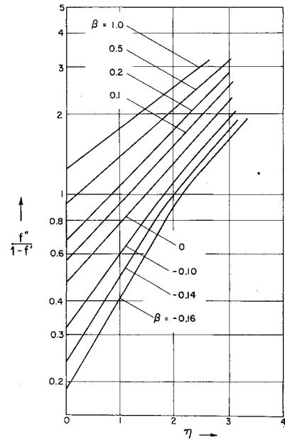
Fig. 1 Local logarithmic decrement in the wedge-flow boundary layer.
